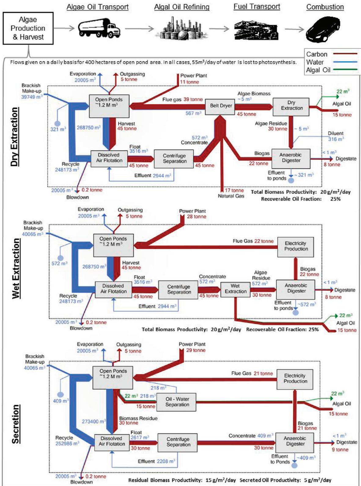
**Figure 2.** Water (m<sup>3</sup>/day) and carbon (tonnes/day) flows in algal oil production for the nominal technology sets. Water consumption in individual process units not included. All flows specific to the 400 ha saline open pond-system modeled; steady state total dissolved solids (TDS) content of 40 parts per thousand (ppt); brackish makeup water with TDS of 20 ppt; evaporation rate of 0.5 cm/day; oil productivity ~2100 gallons/ac/year or 20 m<sup>3</sup>/ha/year.
