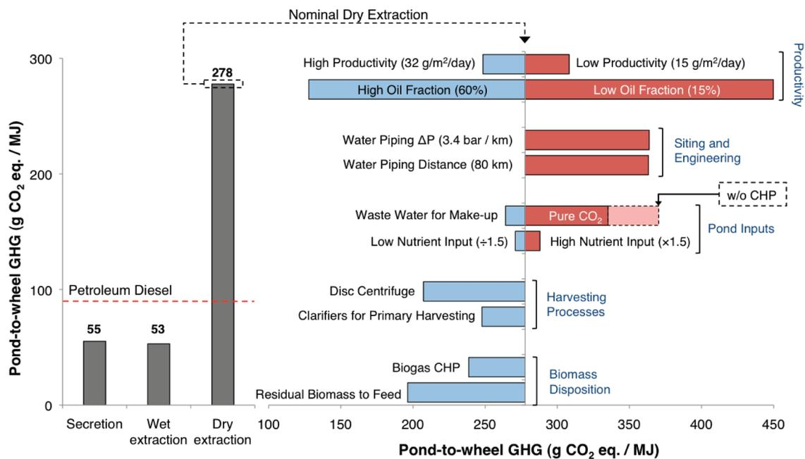
**Figure 3.** Pond-to-wheel GHG estimates for the nominal technology sets (left); parameter/scenario assessment for nominal dry extraction (right). Productivity and process technology assumptions for nominal dry extraction in Table 1. Petroleum diesel value from ref 2. Local sensitivity analysis deemed appropriate because GHG trends largely independent of parameter coupling. Other assumptions and results available as SI; see Sections 4 and 7.
